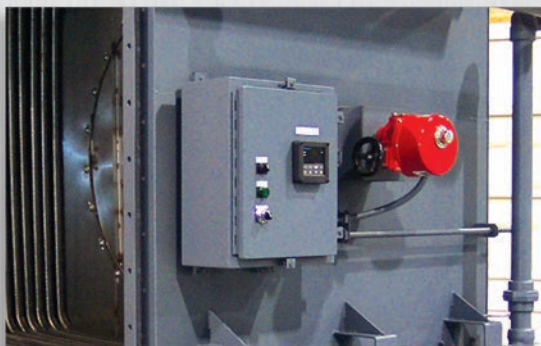
RTR Control panel shown with optional Modulating Bypass Diverter Actuator which powers the diverter to the desired position for maximum heat recovery.
