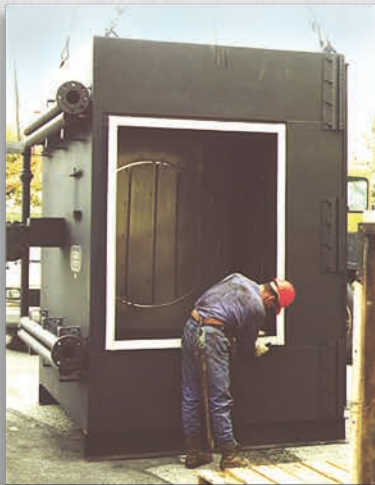
Brewery, Ontario, Canada (1) RTR-1V2Q28CSS recovering Btu from (1) 95,000 pph steam boiler; Reducing 505°F @ 24278 SCFM to 333°F; Raising 196 gpm boiler feedwater entering at 225°F to 278°F.
